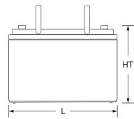
10.19 (259) Ŀ W: 6.61 (168) H: 8.18 (208) HT: 8.42 (214) Tolerances are +/- 0.04 in. (+/- 1mm) and +/- 0.08 in. (+/- 2mm) for height dimensions. All data subject to change without notice.
